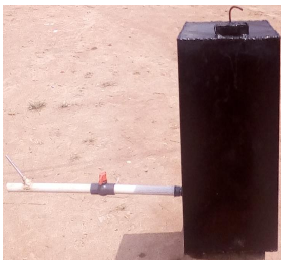
Figure 1. Pictorial Representation of prototype of pressure relief valves system
