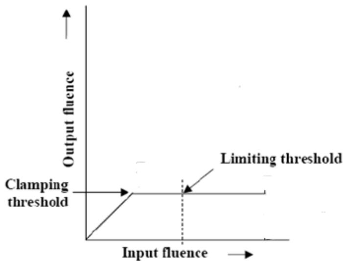
Figure 2. Schamatic representation of the behavior of an ideal optical limiter By plotting of the nonlinear transmittance versus the input fluence as shown in figure (3).
