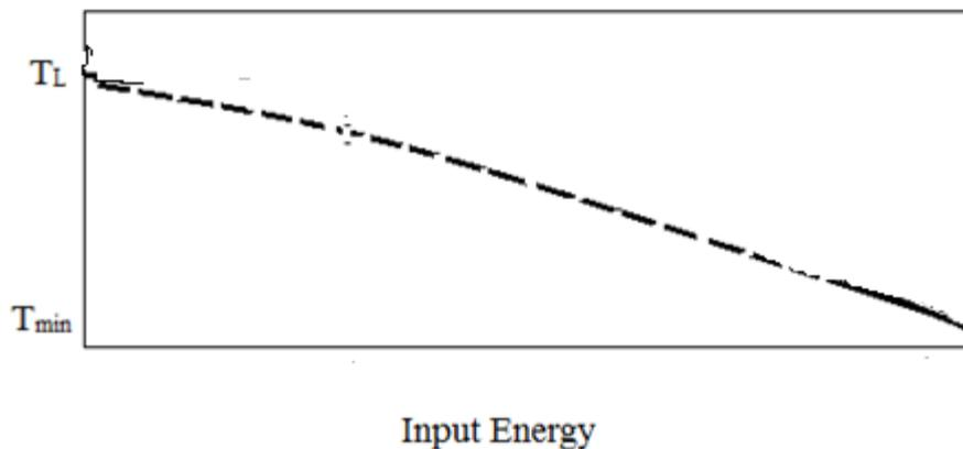
Figure 3. Transmittance output of an ideal optical limiter as a function of the input fluence or energy
