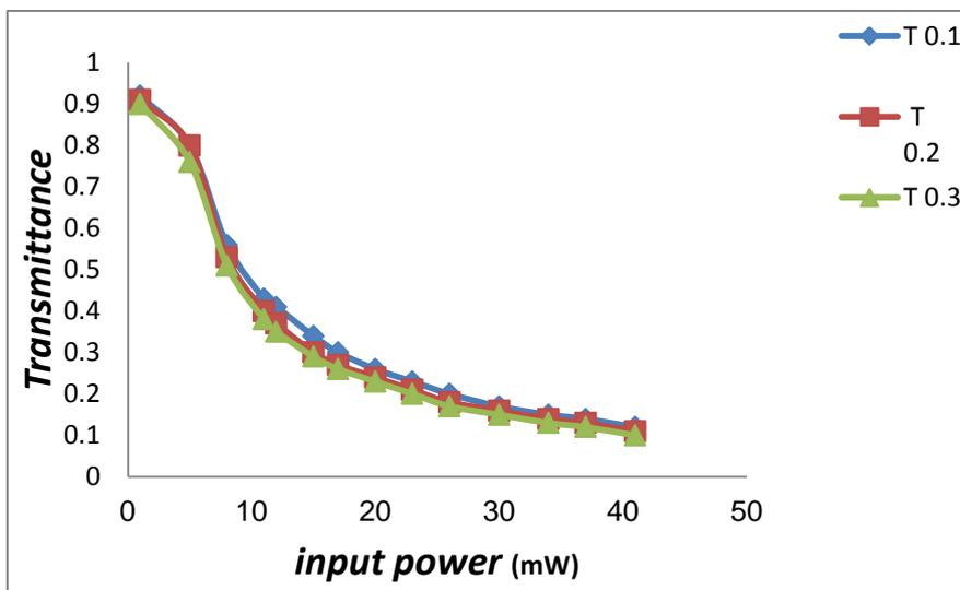
Figure(9): Transmittance output of optical limiter as function of the input power of acridine dye doped Polymer with  $Al_2O_3$  nanoparticles at different weight ratio
