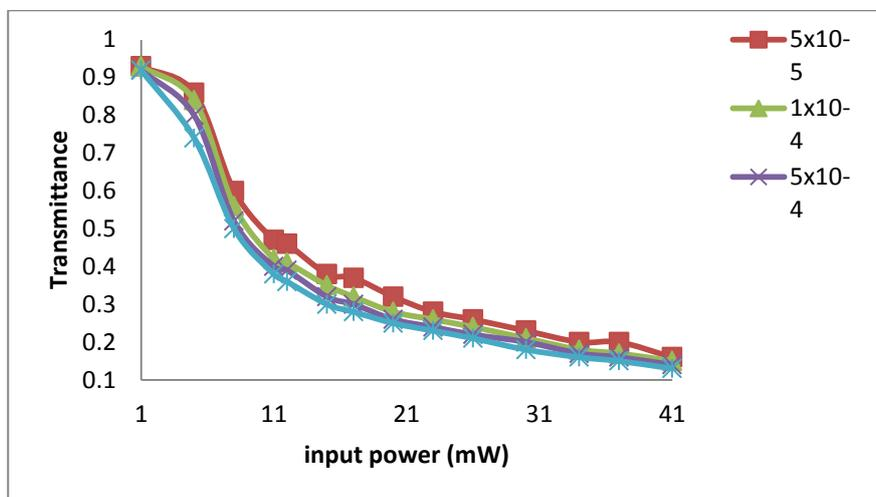
Figure 8. Transmittance output of optical limiter as function of the input power of acridine dye doped PMMA at different concentrations
