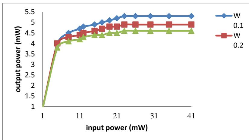
Figure 6. Optical limiting behavior of acridine dye doped Polymer  $Al_2O_3$  with nanoparticles at different weight ratio
