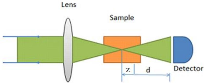
Figure 1. Schematic of the limiting geometry where  $Z$  is the distance between the focal plane in free space and the center of the sample, and  $d$  is the distance from this plane to the aperture plane .
