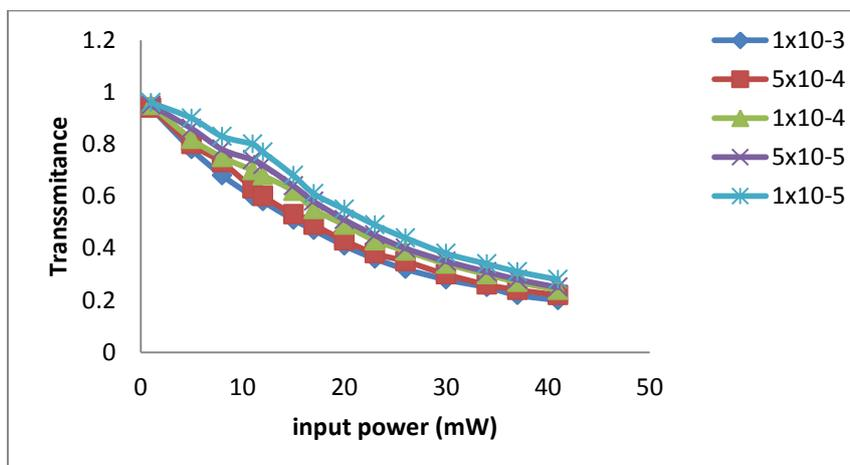
Figure 7. Transmittance output of optical limiter as function of the input power of acridine dye solution at different concentrations
