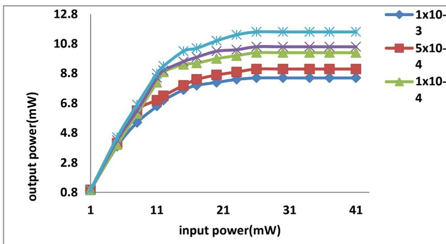
Figure 4. Optical limiting behavior of Acridine dye solution at different concentrations
