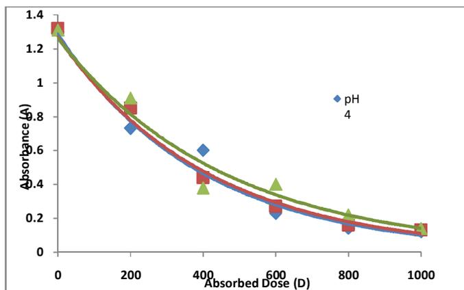
Fig. 2: The exponential decrease in the absorbance (A) with respect to the absorbed dose (D)
