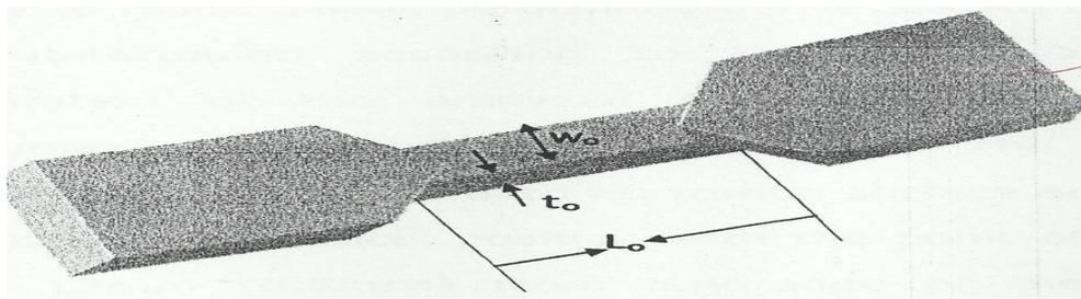
Fig 3.1: Dumbell Shape of Test Sample
