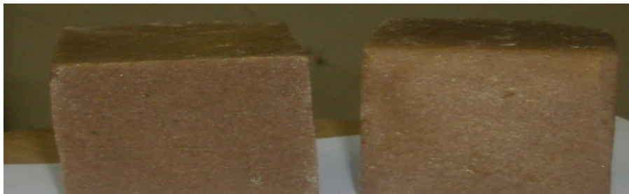
Figure 5. Cubic specimen of polymer concrete
