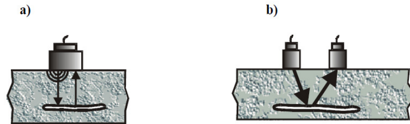
Figure 2. Testing the concrete by ultrasonic echo method: a) transmitting-receiving transducer, b) double transducer
