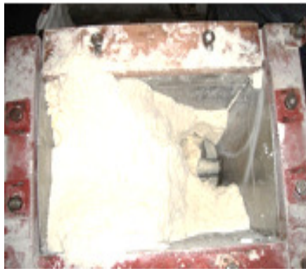
Plate 1: Initial Stage of Rat hole formation Plate 2: Later Stage of Rat hole Formation
