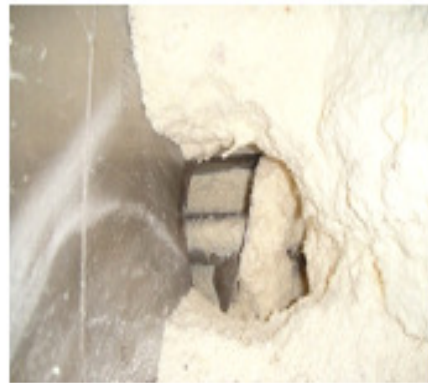
Plate 1: Initial Stage of Rat hole formation Plate 2: Later Stage of Rat hole Formation
