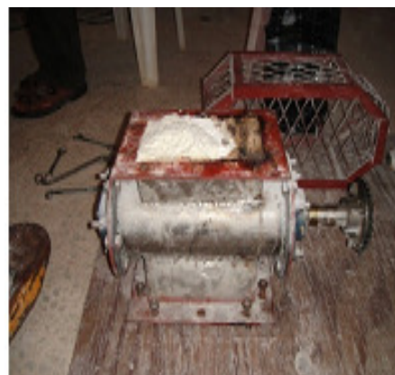
Plate 3: Rotary airlock blocked decayed Plate 4: Rotary airlock with blocked feed with material
