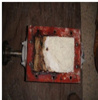
Plate 3: Rotary airlock blocked decayed Plate 4: Rotary airlock with blocked feed with material
