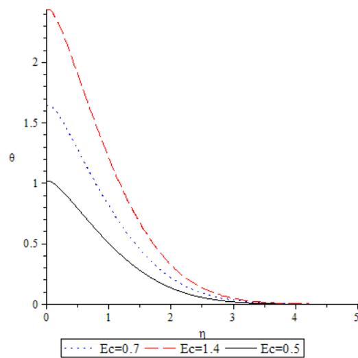
Figure 8: Temperature profile for various values of the Eckert number for  $Pr=0.71$ ,  $Da=0.1$ ,  $H=1$ ,  $G=0.1$ ,  $Bi=0.2$
