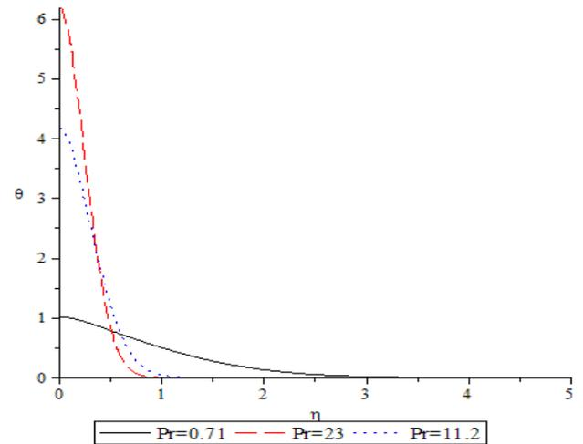
Figure 6: Temperature profile for various values of the Prandtl number for  $G=0.1$ ,  $Da=0.1$ ,  $H=1$ ,  $Ec=0.5$ ,  $Bi=0.2$
