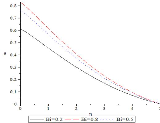
Figure 9: Temperature profile for various values of the Biot number for  $Pr=0.71$ ,  $Da=0.1$ ,  $H=1$ ,  $Ec=0.5$ ,  $G=0.1$
