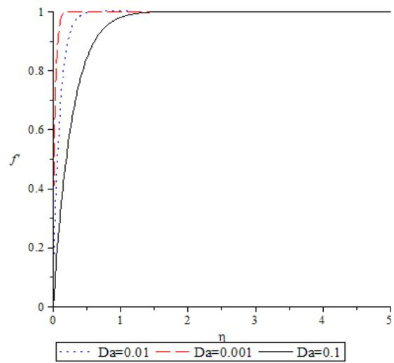
Figure 2: Velocity profile for various values of the Darcy number for  $Pr=0.71$ ,  $G=0.1$ ,  $H=1$ ,  $Ec=0.5$ ,  $Bi=0.2$
