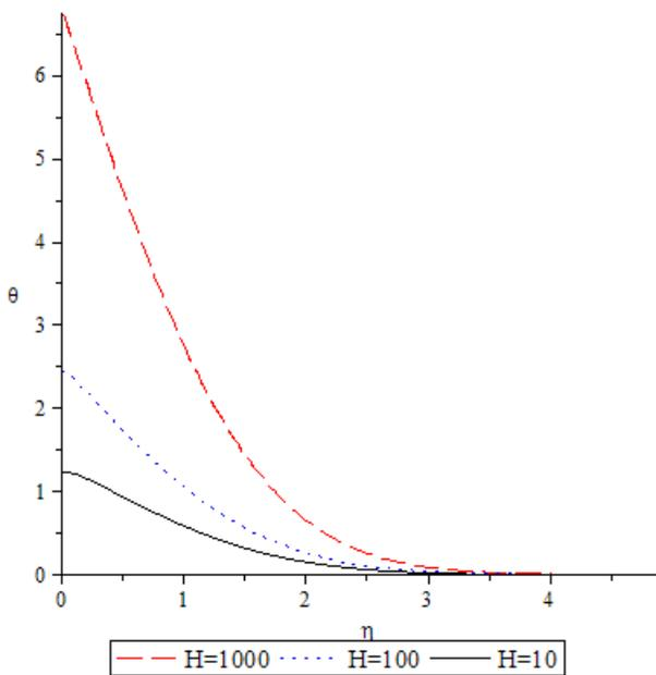
Figure 7: Temperature profile for various values of the magnetic number for  $Pr=0.71$ ,  $Da=0.1$ ,  $H=1$ ,  $Ec=0.5$ ,  $Bi=0.2$
