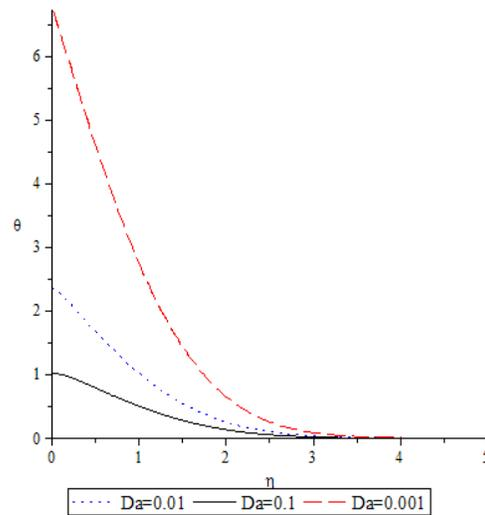
Figure 5: temperature profile for various values of the Darcy number for  $Pr=0.71$ ,  $G=0.1$ ,  $H=1$ ,  $Ec=0.5$ ,  $Bi=0.2$
