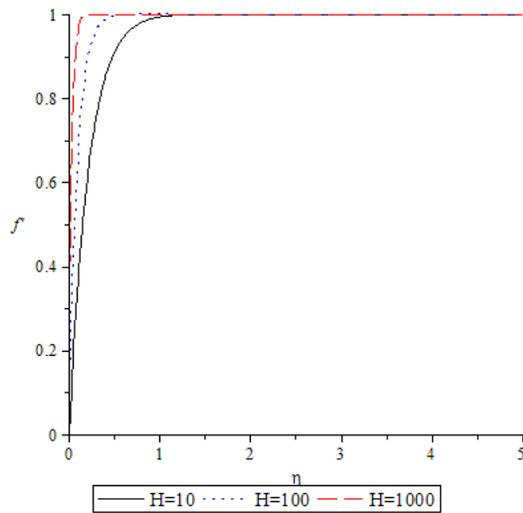
Figure 3: Velocity profile for various values of the magnetic number for  $Pr=0.71$ ,  $Da=0.1$ ,  $G=0.1$ ,  $Ec=0.5$ ,  $Bi=0.2$
