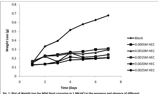
Fig. 1: Plot of Weight loss for Mild Steel corrosion in 1.0M HCl in the presence and absence of different concentration of HEC
