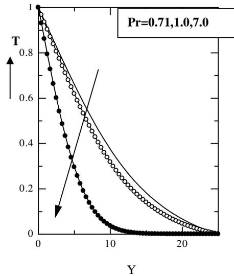
Figure 26. Temperature Profile for different values of Prandtl Number ( $Pr$ ) and  $M = 0.02$  at time  $\tau = 80$
