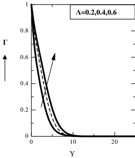
Figure 11. Microrotation Profile for different values of Spin Gradient viscosity parameter( $\Lambda$ ) and  $\Delta = 0.01$ ,  $M = 0.02$  at time  $\tau = 10$
