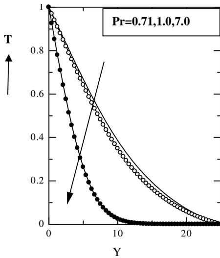
Figure 25. Temperature Profile for different values of Prandtl Number ( $Pr$ ) and  $M = 0.02$  at time  $\tau = 70$
