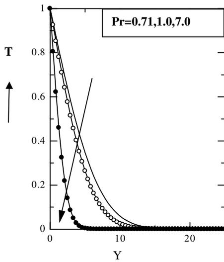
Figure 19. Temperature Profile for different values of Prandtl Number ( $Pr$ ) and  $M = 0.02$  at time  $\tau = 10$
