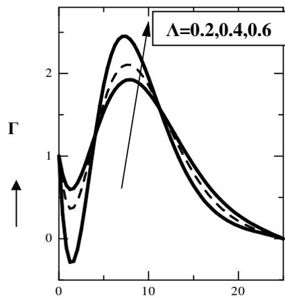
Figure 17. Microrotation Profile for different values of Spin Gradient viscosity parameter( $\Lambda$ ) and  $\Delta = 0.01, M = 0.02$  at time  $\tau = 70$
