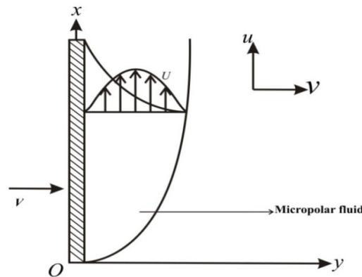
Figure 1. Boundary layer development on a vertical plate
