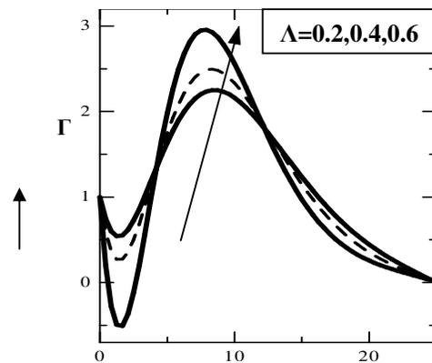
Figure 18. Microrotation Profile for different values of Spin Gradient viscosity parameter( $\Lambda$ ) and  $\Delta = 0.01, M = 0.02$  at time  $\tau = 80$
