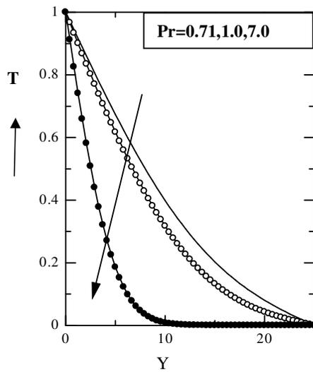
Figure 23. Temperature Profile for different values of Prandtl Number ( $Pr$ ) and  $M = 0.02$  at time  $\tau = 50$
