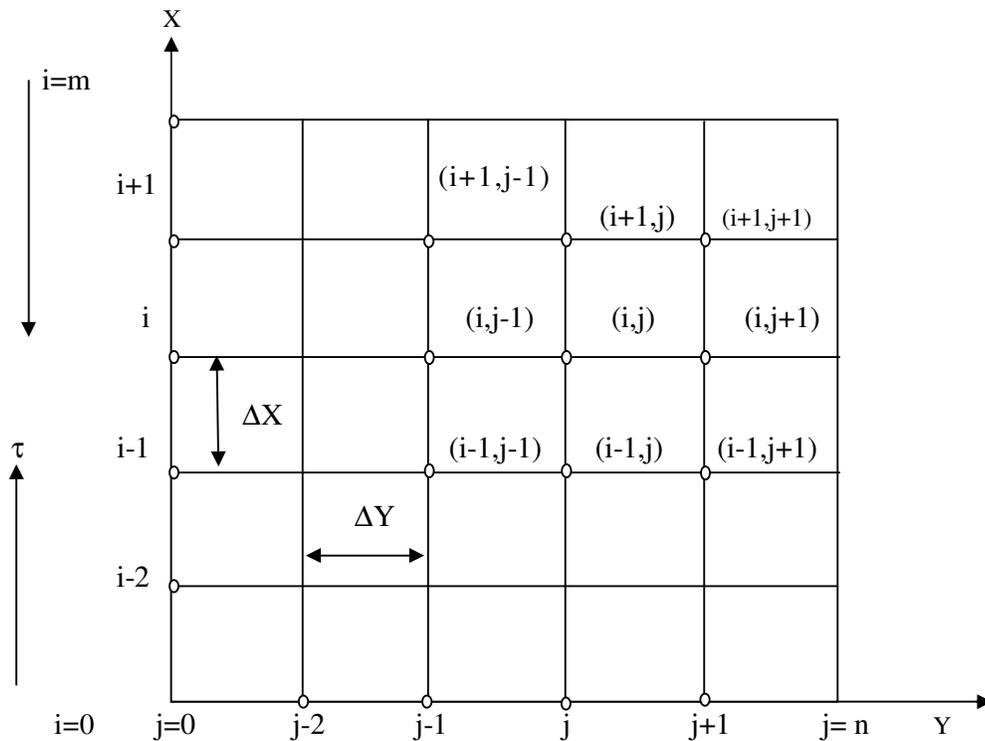
Figure 2. Finite difference space grid.
