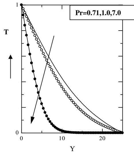
Figure 24. Temperature Profile for different values of Prandtl Number ( $Pr$ ) and  $M = 0.02$  at time  $\tau = 60$
