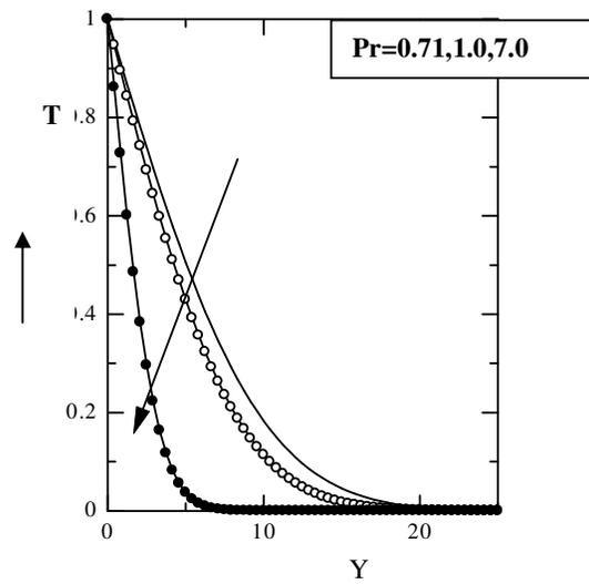
Figure 20. Temperature Profile for different values of Prandtl Number ( $Pr$ ) and  $M = 0.02$  at time  $\tau = 20$
