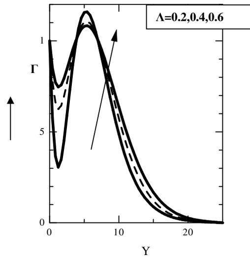
Figure 14. Microrotation Profile for different values of Spin Gradient viscosity parameter( $\Lambda$ ) and  $\Delta = 0.01$ ,  $M = 0.02$  at time  $\tau = 40$
