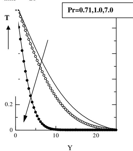
Figure 22. Temperature Profile for different values of Prandtl Number ( $Pr$ ) and  $M = 0.02$  at time  $\tau = 40$
