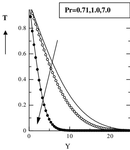
Figure 21. Temperature Profile for different values of Prandtl Number ( $Pr$ ) and  $M = 0.02$  at time  $\tau = 30$
