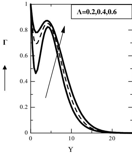
Figure 13. Microrotation Profile for different values of Spin Gradient viscosity parameter( $\Lambda$ ) and  $\Delta = 0.01$ ,  $M = 0.02$  at time  $\tau = 30$
