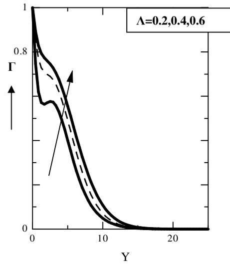
Figure 12. Microrotation Profile for different values of Spin Gradient viscosity parameter( $\Lambda$ ) and  $\Delta = 0.01$ ,  $M = 0.02$  at time  $\tau = 20$
