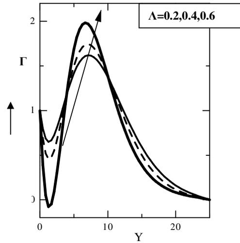
Figure 16. Microrotation Profile for different values of Spin Gradient viscosity parameter( $\Lambda$ ) and  $\Delta = 0.01, M = 0.02$  at time  $\tau = 60$
