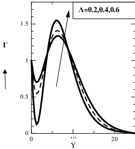
Figure 15. Microrotation Profile for different values of Spin Gradient viscosity parameter( $\Lambda$ ) and  $\Delta = 0.01, M = 0.02$  at time  $\tau = 50$
