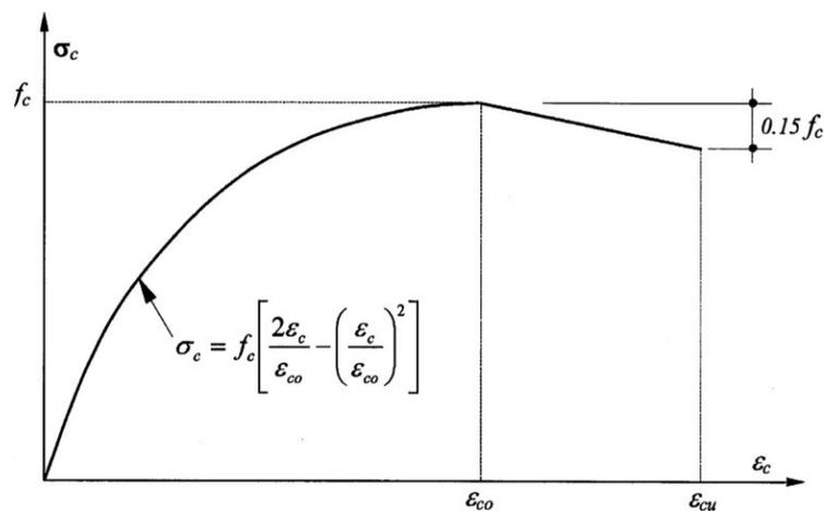
Figure 3. Stress-strain model under monotonic loading (Hognestad, 1951)
