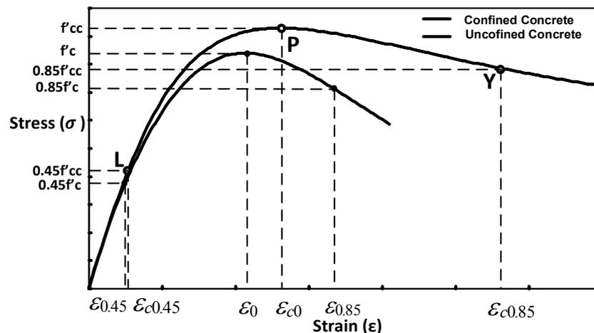
Figure 1. Stress-strain diagram of confined concrete subjected to monotonic loading (Kabir Sadeghi and Nouban, 2010)
