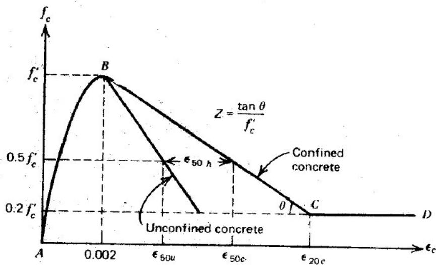
Figure 4. Stress-strain model under monotonic loading proposed by Kent et al. (1972)
