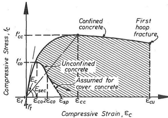
Figure 2. Stress-strain model for monotonic loading (Mander et al., 1989)
